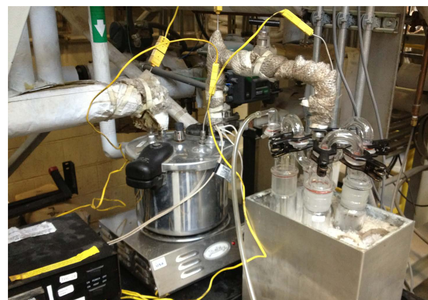
Figure 3. Collecting liquid samples of nitrogen compounds using glass impingers downstream of tar condensing pressure cooker.
